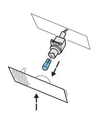
4. Remove the bulb socket by turning it counterclockwise and pulling it straight out.
